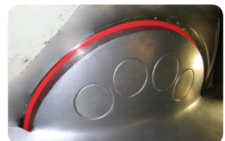
Step 6: Installed seals for runner blades
