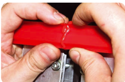
Step 4: Visual inspection of weld
