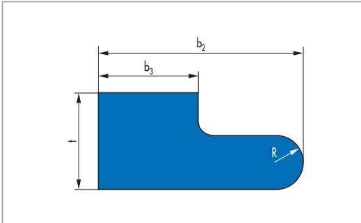
Mating rings are used for fastening and prevent axial movement of the U-rings, which can damage the sealing edges at the sealing lips. They are manufactured using extruders. The mating rings are always supplied by the metre.
