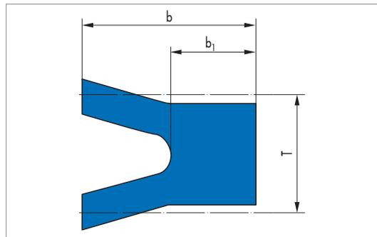
U-rings are produced, extruded and bonded to the butt for use as piston or rod seals. U-rings made of NBR and FKM are also available with vulcanisation to butt. They can be supplied at extremely short notice.
