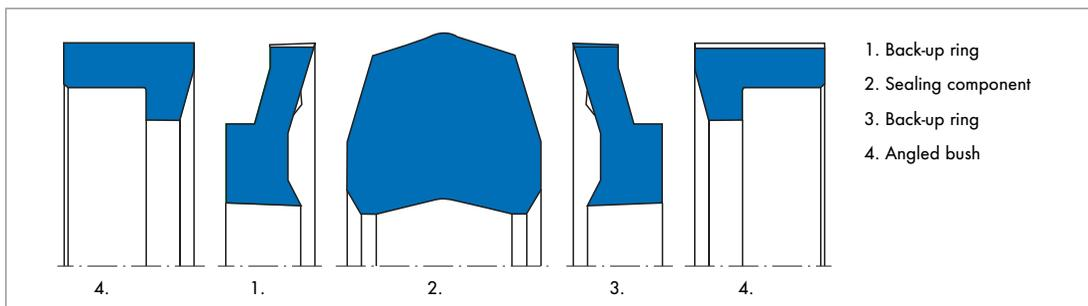
Fig. 52 Fitting of Merkel Compact Seal L 43
