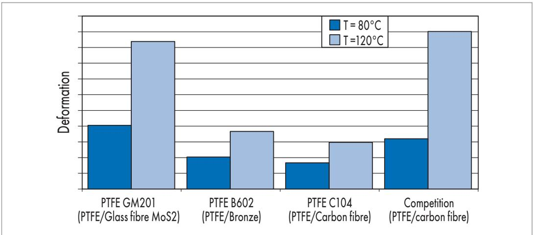
Fig. 34 Form stability of PTFE compounds in comparison
