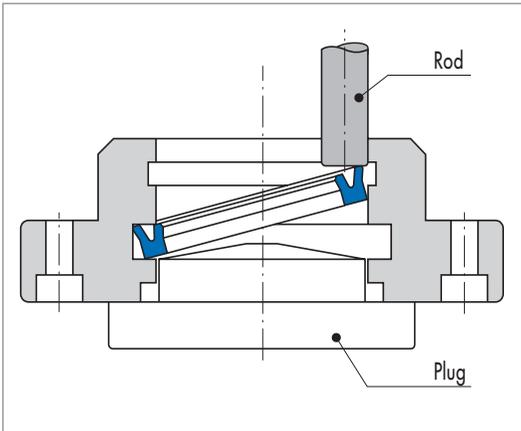
Fig. 41 Installation aid for rod seals
