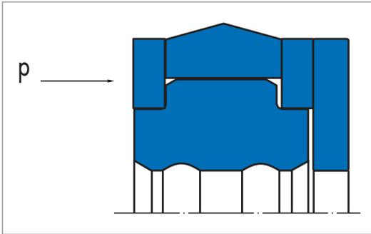
\* If a full-surface back-up ring is used on the side not subjected to high pressure, the use of up to 150 MPa is possible. The height of the backup-ring should be 5 mm.
