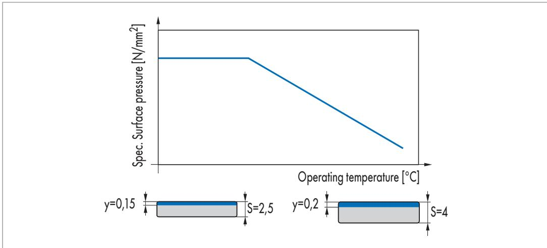
Fig. 13 Deflection at maximum surface pressure
