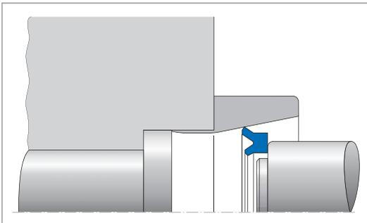
Fig. 42 Fitting of rod seals in divided housings
