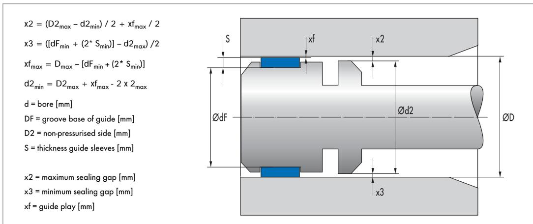
Fig. 23 Limit values of sealing gap of piston sealing system
