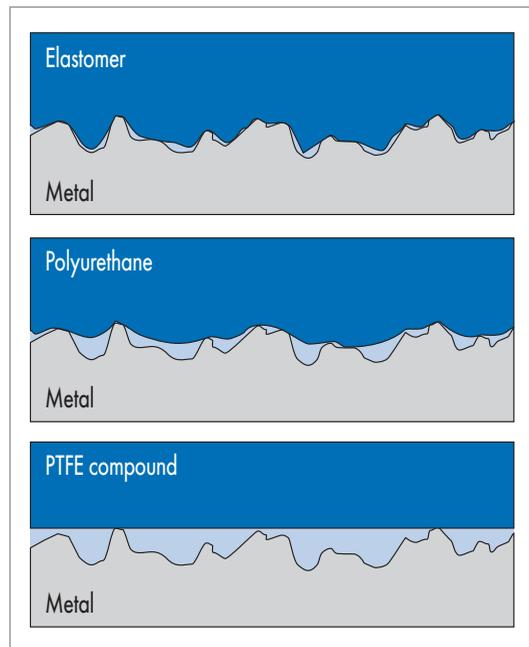
Fig. 33 Sealing edge in contact with counter surface
