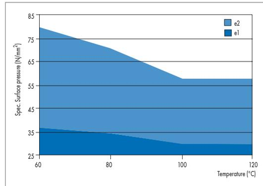
Special surface pressure for parallel load
