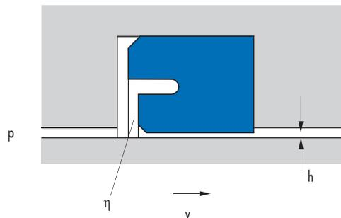
Fig. 15 Compression curve and hydrodynamic lubrication film formation
