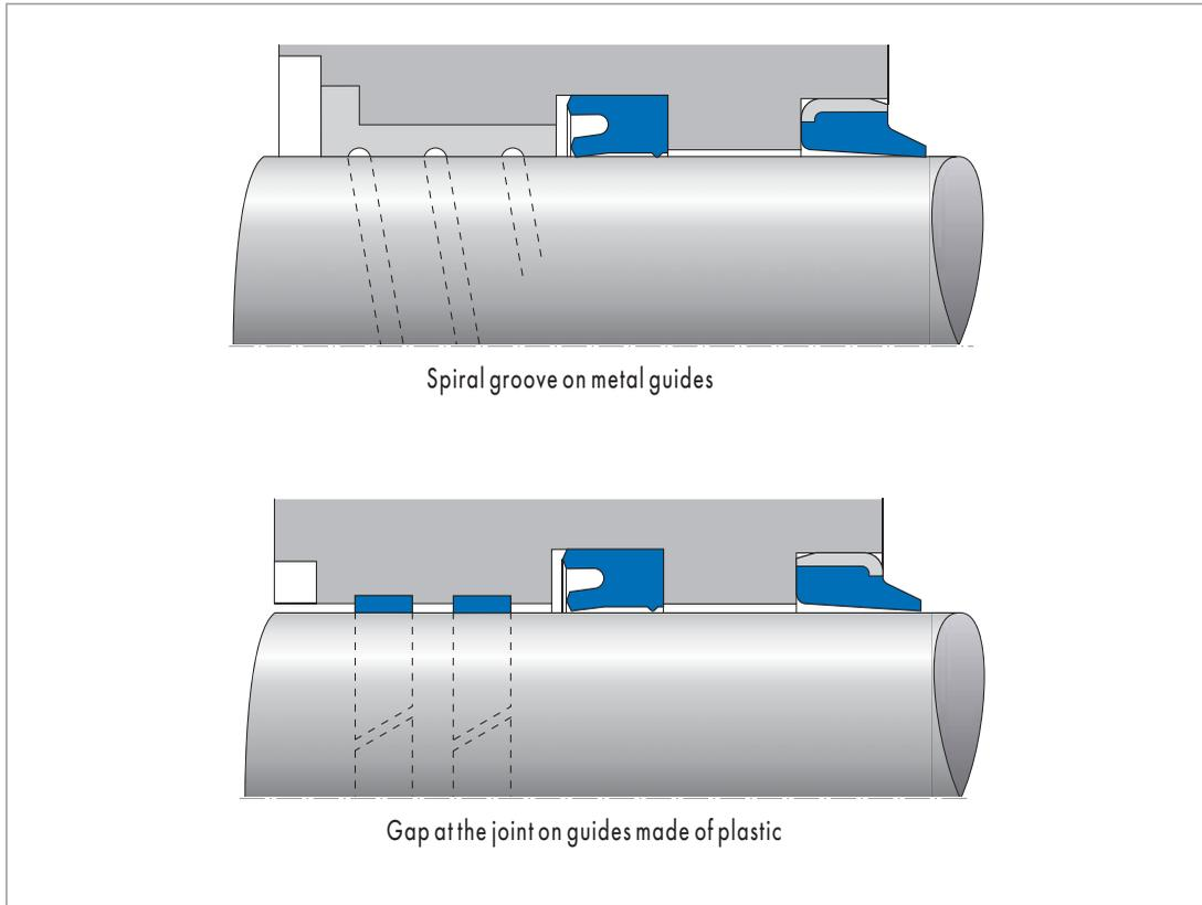
Fig. 19 Design measures for preventing drag pressure
