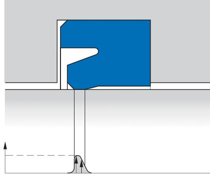
Contact pressure distribution as a result of initial compression
