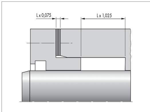
Adjustable housings have the advantage of an optimal adjustment option for the sealing effect with minimal idling friction. After a lengthy period of running and incipient wear on the seal tightening the gland can extend the durability and significantly delay a system standstill. For adjustable housings an extension of 2,5% and an adjustability of 7,5% of dimension L is recommended. Non-adjustable housings have the advantage
