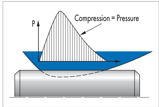
Fig. 26 Qualitative compression curve, single-acting rod seal
