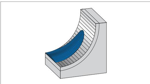
Fig. 9 Guide ring with convex profiling
