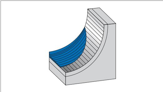
Fig. 8 Guide ring of fabric-base laminate
