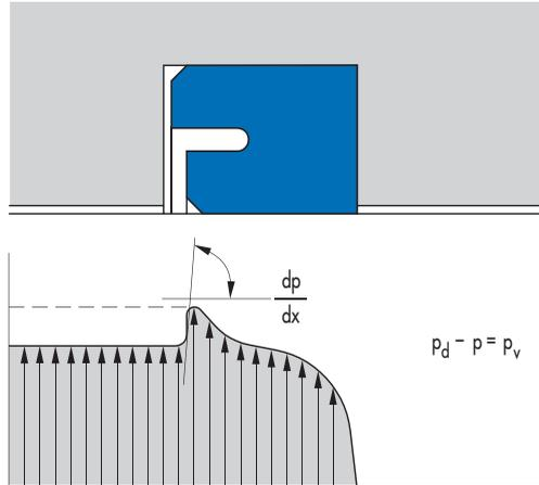
Contact pressure distribution as a result of initial compression and pressure to be sealed
