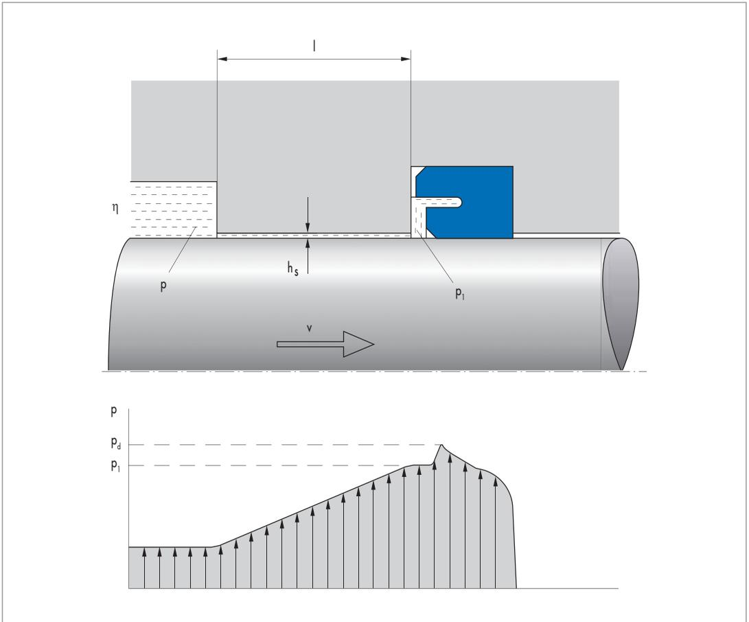
Fig. 17 Hydrodynamic drag pressure
