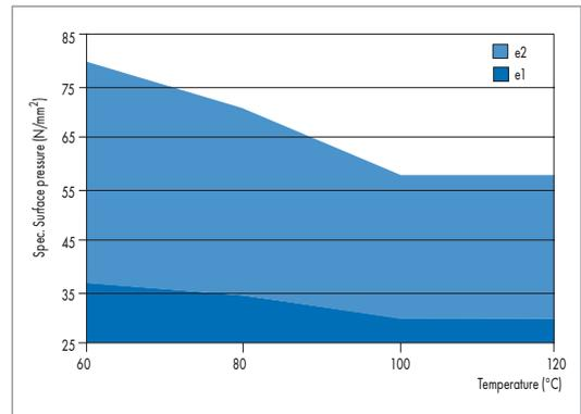
Special surface pressure for parallel load
