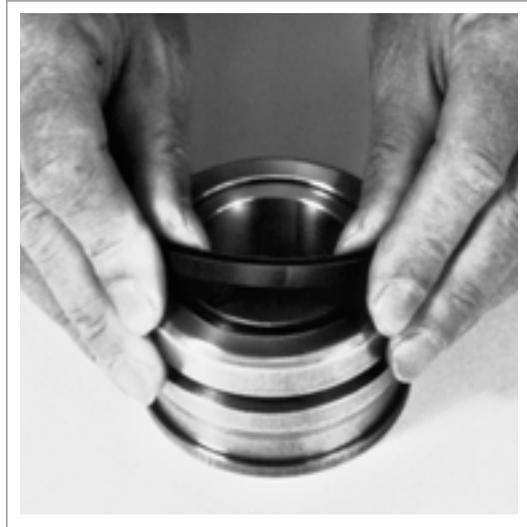
Fig. 43 Snapping in the polyurethane running ring
