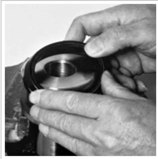
Fig. 46 Inserting sealing ring
