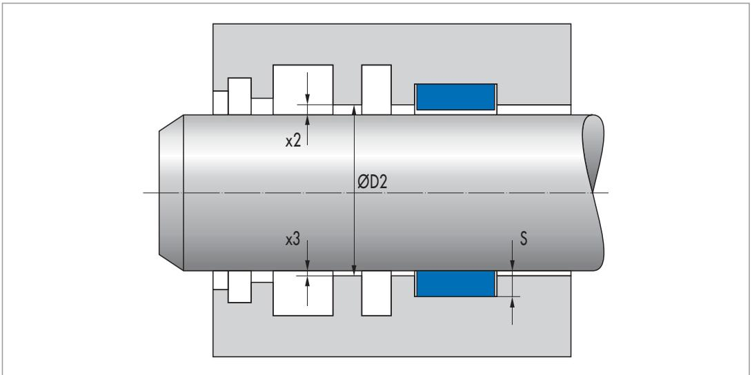
Fig. 14 Sealing gap
