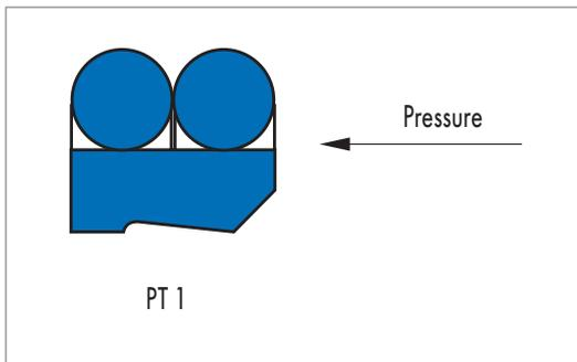
Fig. 53 Functional direction of wiper
