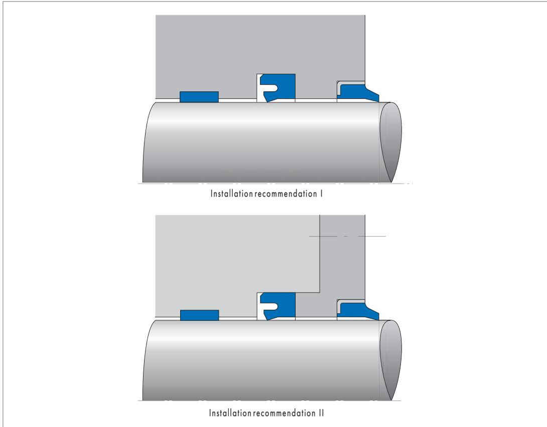
Fig. 38 Installation types of rod seals
