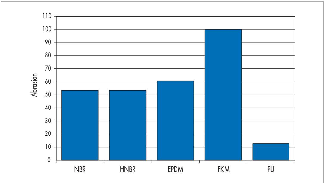
Fig. 35 Wear behaviour in comparison
