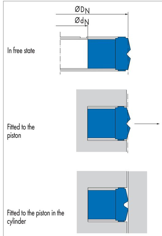
Fig. 3 Piston seal
