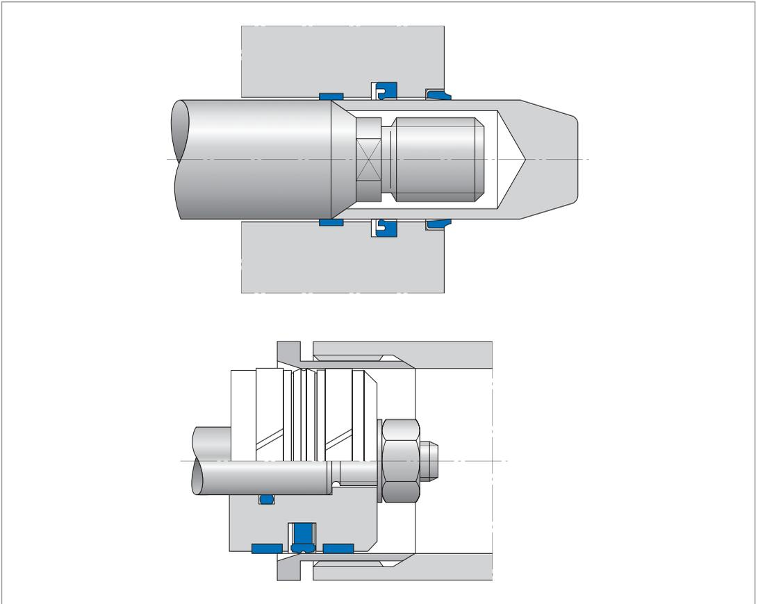
Fig. 37 Covering threads when mounting seals
