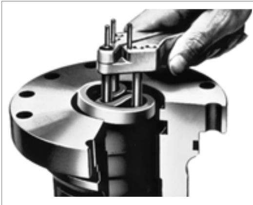
Fig. 39 Fitting tool I for rod seals
