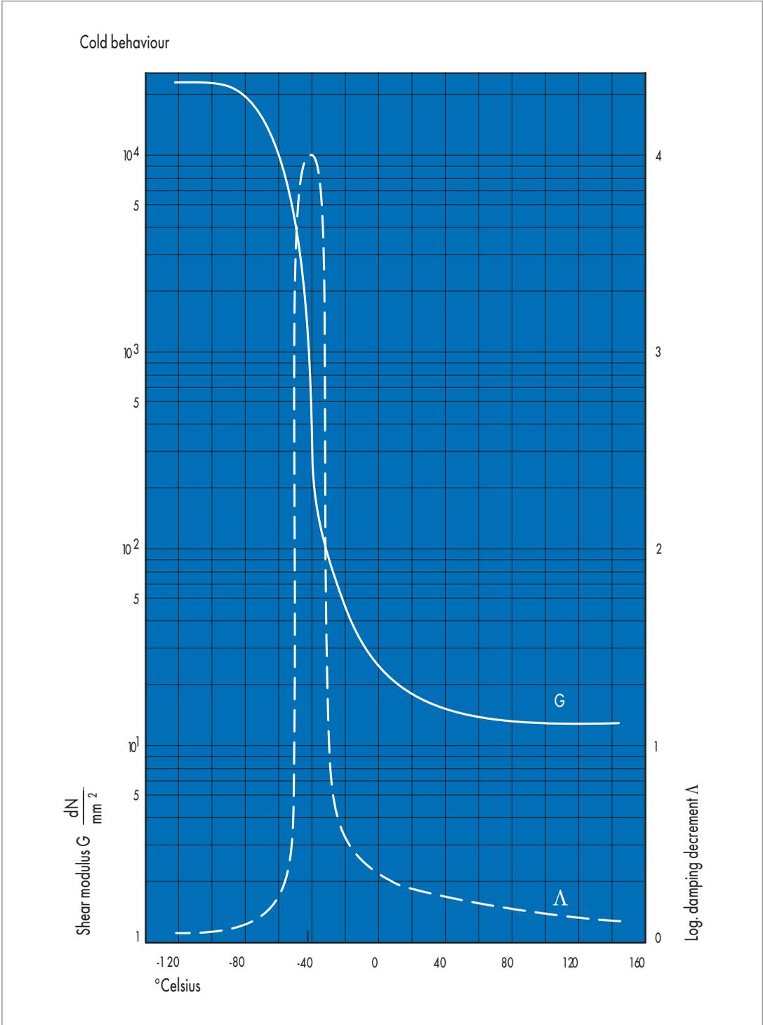
Fig. 20 Graph: torsion vibration test in accordance with DIN 53445; dynamic shear modulus G and logarithmic decrement Δ of a Simrit material based on CR
