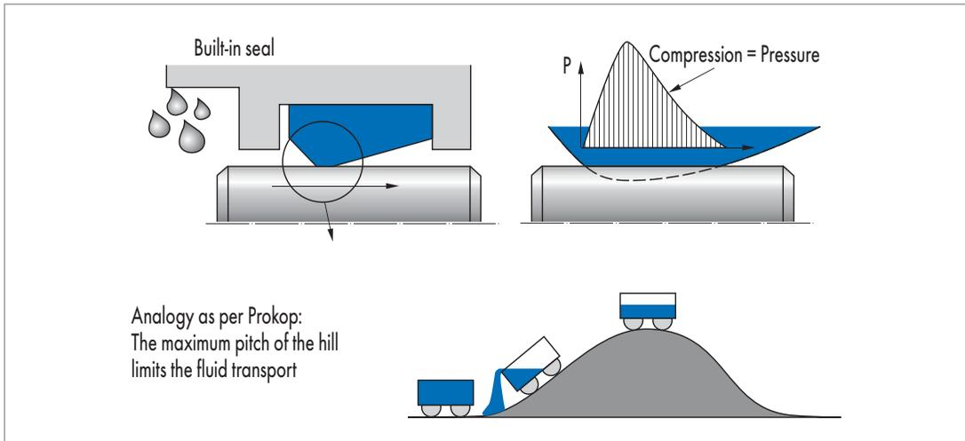
Fig. 5 Qualitative compression curve, single-acting rod seal
